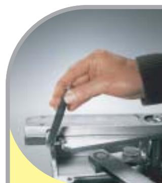
*Simple and safe unlocking system by special key.*
